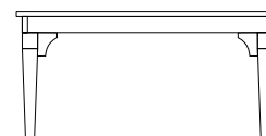
BUNGALOW CHAT TABLE, 40X40 FINISH: PERDIDO TOP: ALUMINUM SLAT 40"W x 40"D x 20"H APRON: 16.8"H | INSIDE WIDTH: 33.6"W 5100040-0105000
